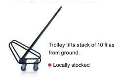
Trolley with welded mild steel tubes and bars, finished in a black epoxy powder coating. Castors with nylon hub and rubber wheel (75kg rating each).
